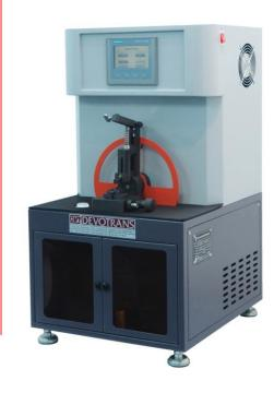
Used to determine strength of  $\emptyset$  0.3 mm – 2.5 mm metal wires to plastic deformation when subjected to 90° bending.
